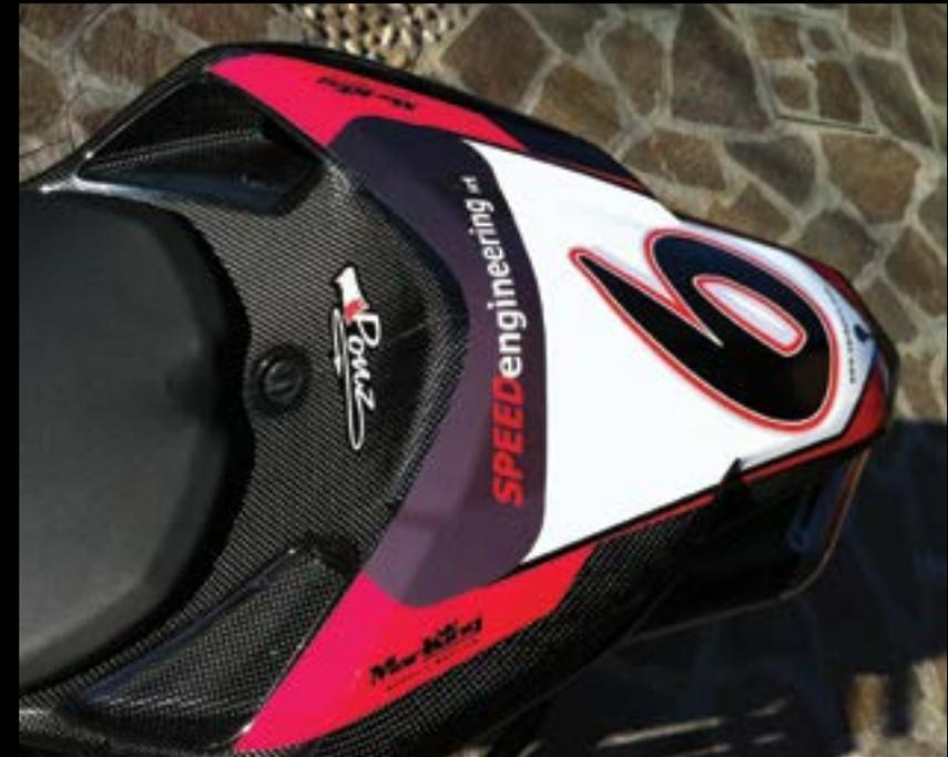
Carbon fibre single race seat with Carbonin decal design
