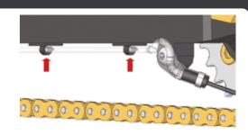
Cable Ties (part 12) can be used to secure vacuum tubing to existing wiring or to the frame or sub-frame to route neatly to the RMV. Take care not to pinch the tubing by over tightening. continued over
