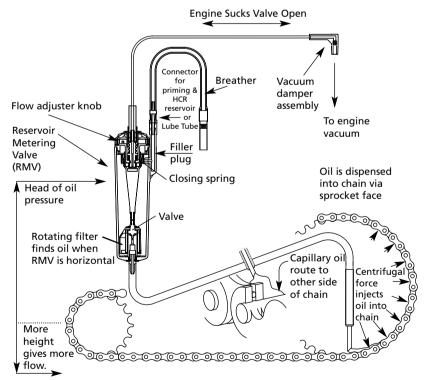
How does the Scottoiler work? The Scottoiler vSystem is vacuum operated. When the motorcycle engine is running vacuum is generated, this lifts a diaphragm which in turn opens the valve. Whilst open the valve allows oil to drip feed under gravity down the delivery tube to the chain via the rear sprocket. There is metering built into the valve to provide adjustment to control the rate at which oil is dispensed. It is not a pump.
