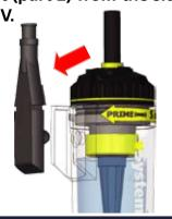
Fit the spout to the bottle of Scottoil and fill the RMV though the hole in the side of the reservoir.
