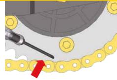
Hint: Nib should be touching sprocket with slash cut facing out.
