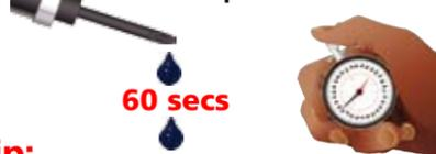
**Top Tech Tip:** For best results, clean the chain thoroughly with paraffin and a nylon brush. Manually drizzle Scottoil along the length of the chain and wipe off any excess. The flow from the RMV then simply tops up this initial coating.
