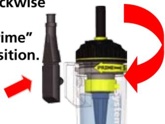
Connect the spout to the Filler Plug. Squeeze the bottle of oil to pressurise the system. This will force oil down the delivery tubing. Squeeze until there are no bubbles.
